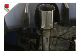
A) Remove the valve motor from the original exhaust.
